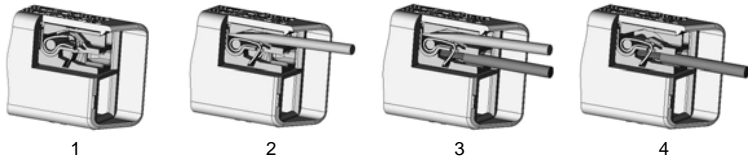
Figure 7-2: Cable connection to screwless terminals
