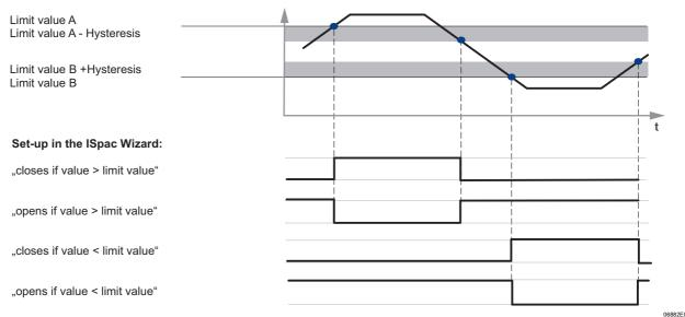
In case of a detected line fault, the limit value relays adopt the set operating direction, for example, in case of "Off above limit value", the relays drop out. This is the recommended setting for safety-related circuits.
