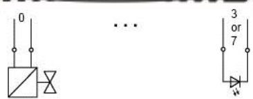
Approved intrinsically safe solenoid valves, indicating lamps
