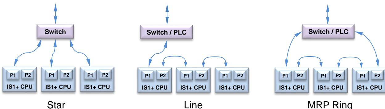
**Maintenance Note:** The internal switch and the Port P2 of a 9442 CPU are disabled during a software update. Following Network participants connected on port P2 are therefore unavailable in this phase of the operation.
