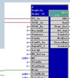
Driver for PCS7 V9 based on IS1+ GSDML-V2.34-Stahl-RIO9442-20200427.xml supports IS1+ CPU 9442 with PROFINET S2 redundancy.
