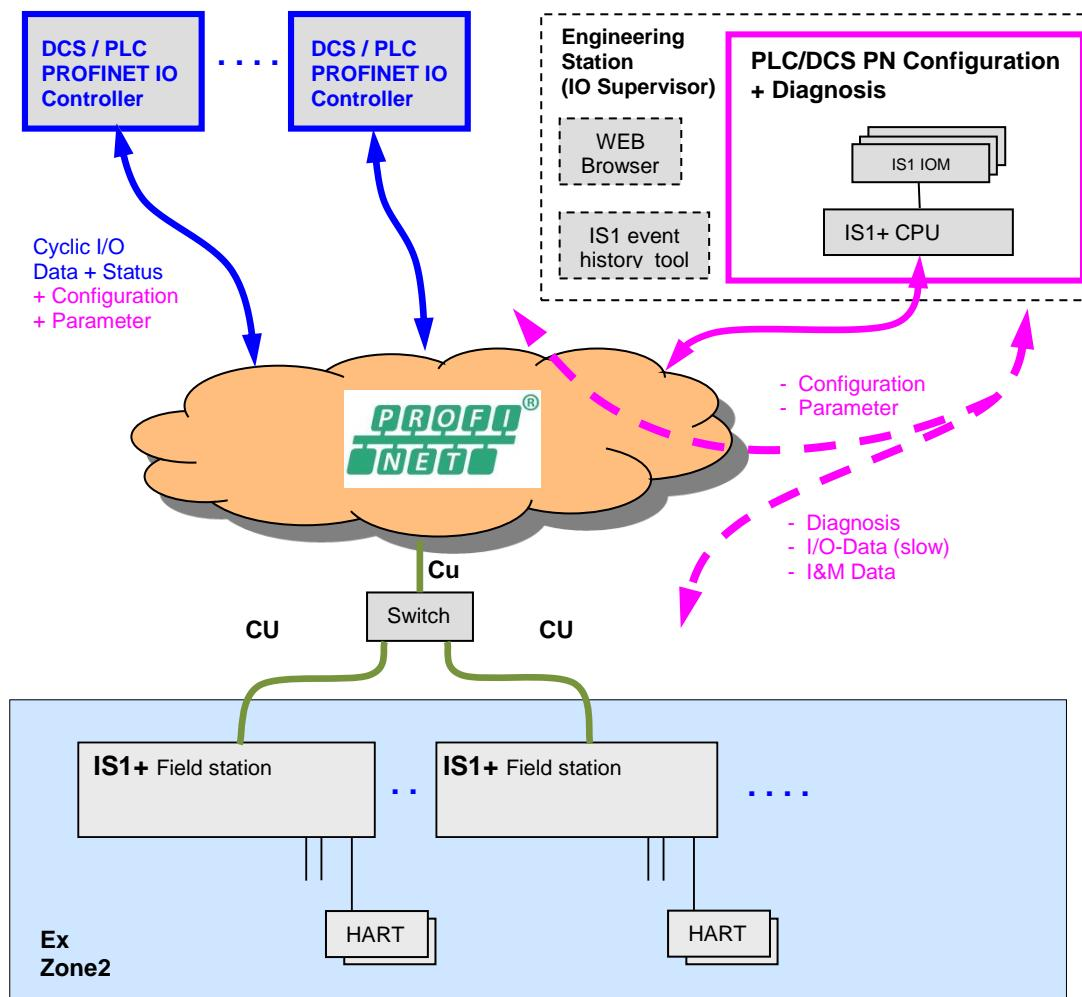
As an off-the-shelf explosion protected unit, the IS1+ field station can be installed directly in the potentially explosive atmosphere (Zone 1 or Zone 2). It can also be installed in the safe area. The diagram above shows a Zone 2 solution.
