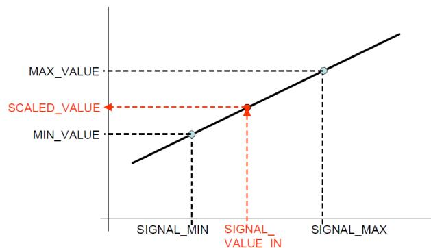
$$\text{SCALED\_VALUE} = (\text{SIGNAL\_VALUE\_IN} - \text{SIGNAL\_MIN}) \frac{(\text{MAX\_VALUE} - \text{MIN\_VALUE})}{(\text{SIGNAL\_MAX} - \text{SIGNAL\_MIN})} + \text{MIN\_VALUE}$$
