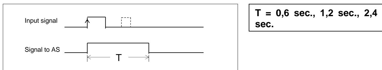
Pulses which are longer than the parameterized time  $T$ , are not extended.
