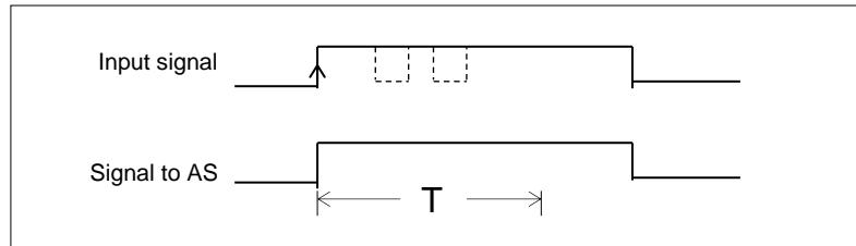
**Pulse extension with inverted operation:**
