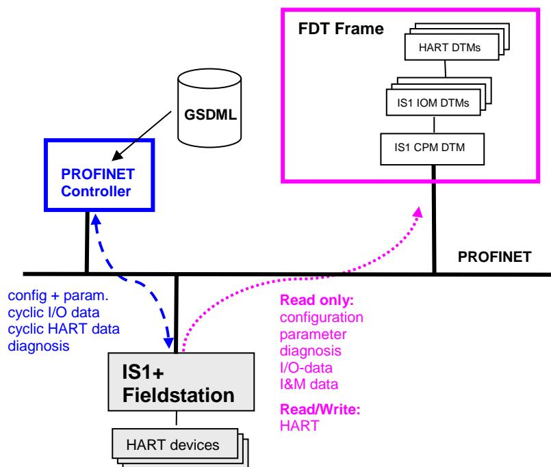
Configuration and parameterisation of the IS1 fieldstation shall be done with the PROFINET controller using GSDML.
