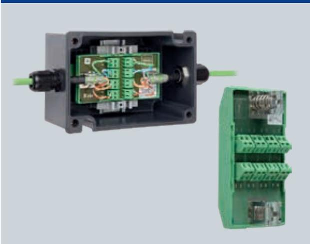
The 8187 Ethernet terminal is used to connect CAT5/6/7 cables with transmission rates of up to 1 GBit/s in Zone 1 hazardous areas.
