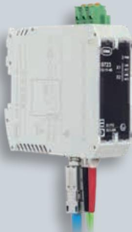
The Ethernet media converters for installation in Zone 1 convert Ethernet via fibre optics (FX) to Ex i Ethernet via CAT cable (TX). With this converter, industrial CAT cables can be plugged and unplugged during operations also in Zone 1 (hot plug). The devices are particularly suitable for operation of the Zone 1 Remote I/O IS1+.
