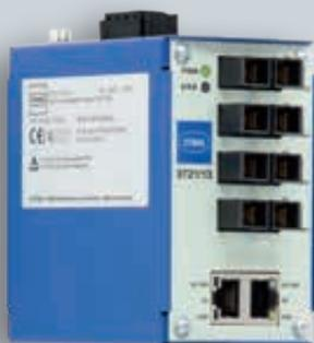
The 9721 switch is used for linking electrical Ethernet networks with optical 100 Mbps Ethernet networks. With type of protection "op is", the 4 FO ports are designed for operation in hazardous areas (see IEC EN 60079-28). This way, conventional fibre optic cables can also be used in hazardous areas and may be connected and disconnected during operation (hot plug).
