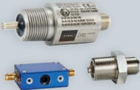
The 9730 series HFisolator from R. STAHL, which can easily be connected between a wireless device and an antenna, converts the radio signal into an intrinsically safe (Ex i) signal. R. STAHL offers two versions of this device, as a simple signal converter or a combined signal converter and enclosure feed-through.
