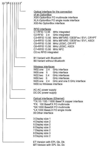
In the complete type designation, the asterisks are replaced by alphanumeric or symbolic characters to indicate different variations of the apparatus without relevance for explosion protection.
