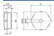
$\begin{array}{ll} \text{M = Thread size} & \text{d = Width across corners} \\ \text{h1 = Thread length} & \text{h2 = Dimension h2} \\ \text{SW1 = Hexagon socket width across flats} \\ \text{SW2 = Width across flats} \end{array}$
