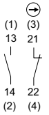
Schaltbild 8003/143 NC positive opening / NO Numbers in brackets according to core identification
