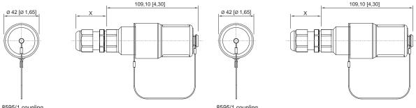
8595/1 coupling X = depending on the cable gland used 8595/1 coupling X = depending on the cable gland used
