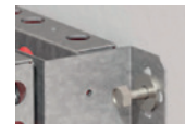
Sandwich design Insert 4 x M6 screws and washers in the mounting brackets as shown. Use a wrench for tightening the screws firmly.
