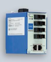
The switch 9721 is used for linking electrical Ethernet networks with optical 100 Mbit/s Ethernet networks. The 4 FO ports are designed for operation in the hazardous areas with the "op is" type of protection. This way, conventional fibre optic cables can also be used in hazardous areas and may be connected and disconnected during operation (hot swap).
