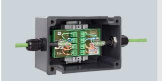
Ethernet terminal 8187 is used to connect CAT5/6/7 cables with transmission rates of up to 1 GBit/s in Zone 1 hazardous areas and replaces the not permitted industrial connectors.
