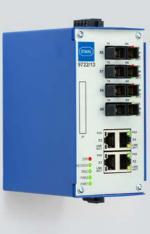
The managed 100 Mbit/s switches series 9722 are specifically designed for use in PROFINET networks. They feature ring functionality based on the Media Redundancy Protocol. The 4 FO ports are designed with the "op is" type of protection, making maintenance of the devices in Zones 0, 1 and 2 easy (hot swap, hot plug).
