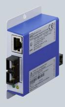
The media converter series 9721 converts electrical signals into inherently safe optical "op is" signals, allowing installation and maintenance work to be conducted on fibre optics in Zones 0, 1 and 2 without the need for downtime (hot swap/hot work). It is particularly suitable for the Ethernet remote I/O system IS1+.
