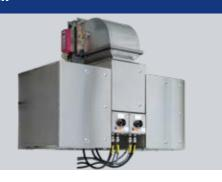
A Fan Box is a ventilation system designed to obtain an overpressure inside a room or containerized solution. It is equipped with its own control system, executed in a CUBEx series 8264 enclosure. For more reliability the ventilation system can be redundantly executed.
