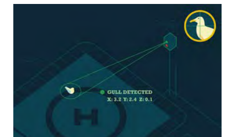
The system determines the exact location of the bird and fires a targeted laser
