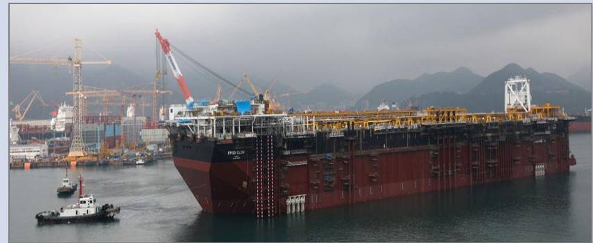
Example of a Floating Production and Offloading Unit (FPSO)
